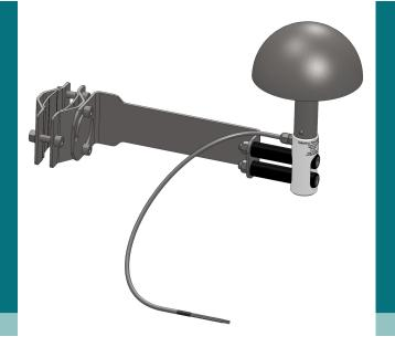
The RHD is a low-cost, high precision, ultra-robust rain gauge. It features very low-power consumption, is maintenance- free and has a completely sealed acoustic sensor with no moving parts. The sensing device is a polished stainless steel hemisphere supported by a strong stainless steel arm. It detects changes of the acoustic pressure that are induced by the impact of raindrops or hailstones. The RHD also includes a distrometer that return the drop size distribution.
