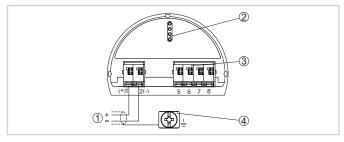
Secondary terminal connections (intrinsically safe devices)
