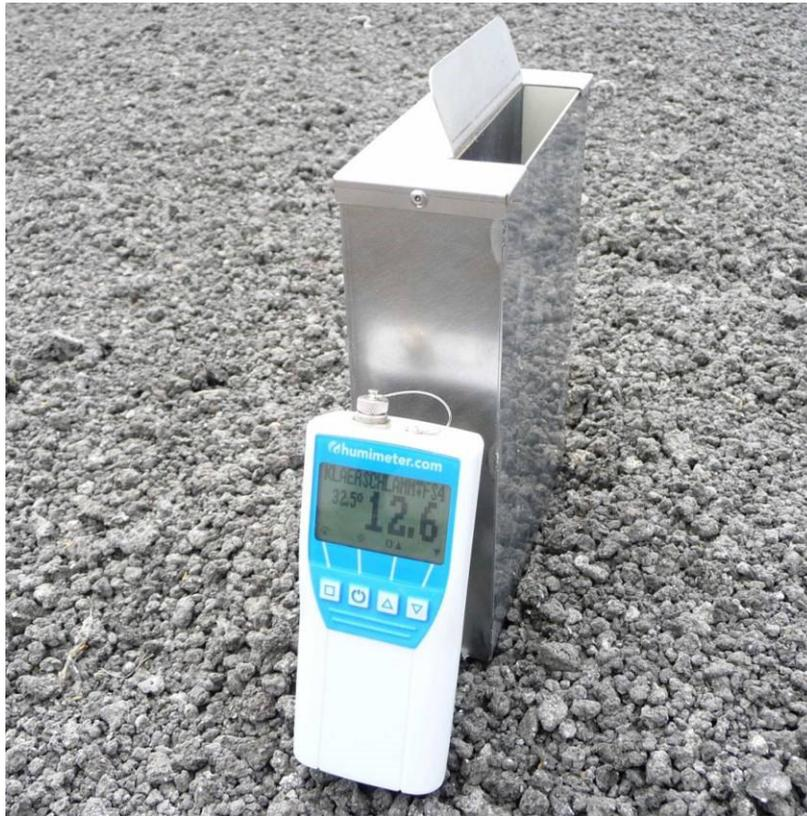
Sludge granulate moisture meter
