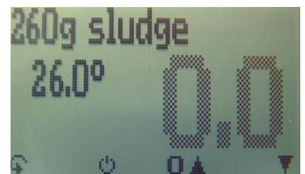
6. Fill up the cup with the sample material (+/- 1.0g). **The fill quantity is shown on the upper left corner on the display of the humimeter.**
