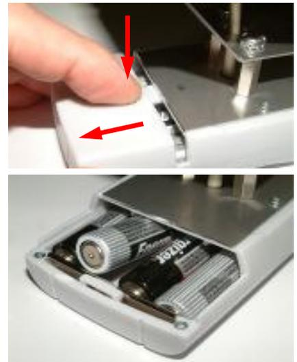
If the battery symbol appears in the measuring window resp. if a critical charge of battery is shown in the status, the batteries have to be changed IMMEDIATELY.
