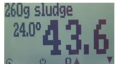
9. If the measure value is blinking, the valid measuring range is exceeded (limits see list on page 5). In this case the accuracy will be decreasing.
