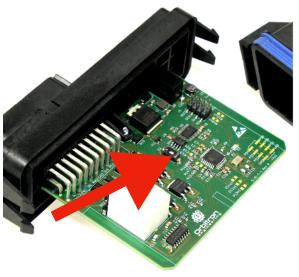
You will find a switch (red arrow) in the very middle of the circuit board. With a simple toggle CAN termination can be turned off.
