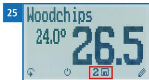
» The display will now appear as shown in figure 25. The marked number shows the number of readings that have already been saved.
