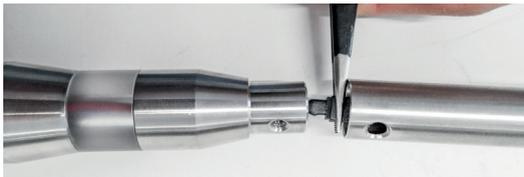
Now carefully insert the measuring tip into the tube. Now align the measuring tip by twisting it so that the holes match in order to attach the screws.
